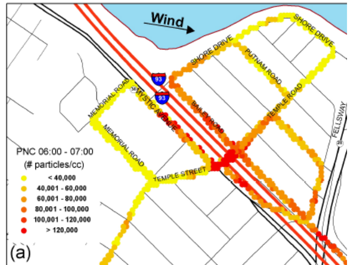
Figure 6 Plots of data from a mobile monitoring trips near I-93 in Somerville. Darker red indicates higher concentrations of UFP. Source: Durant, 2010; Padró-Martínez, 2012
