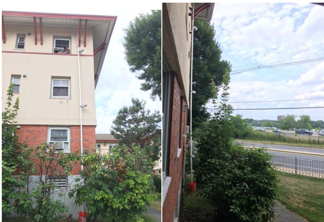
Figs 10(a) and (b)- REED-4023 SLMs at 5 ft, 15 ft and 25 ft (I-93 SB traffic visible at right)
