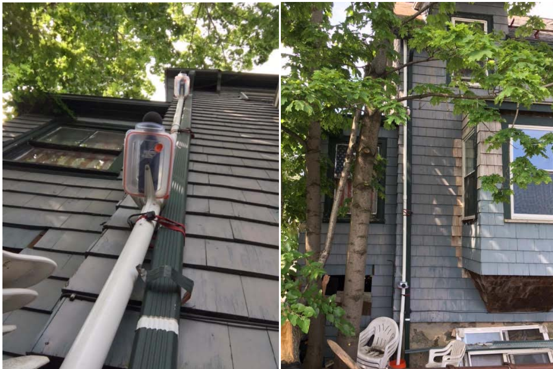
Figures 6(a) and (b)- REED-4023 SLMs Deployed at 5 ft and 15 ft (25 ft not deployed)
